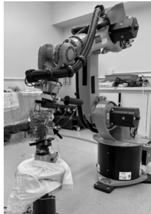
Fig. 6. Example setup of the robotic testing system for biomechanical validation of the 360° lumbar arthroplasty construct.
