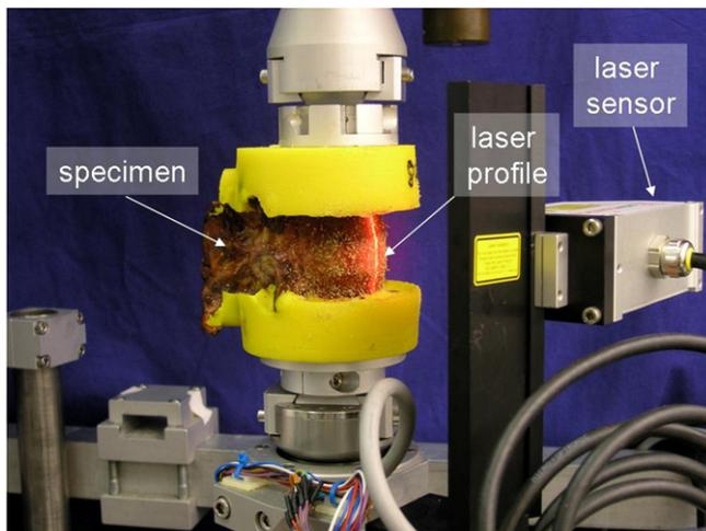
**Fig. 1.** Six L2–3 specimens were loaded in the spine tester with pure bending moments of 7.5 Nm. Surfaces of the specimens were obtained with a custom-built laser scanning system. This laser scanner rotated about the specimen while it acquired the spatial data within a single turn. Surface data were assessed for all loading directions including axial compression, flexion, extension, lateral bending and axial torque.
