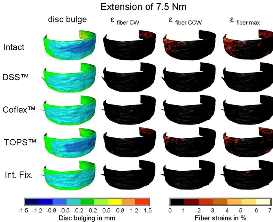
**Fig. 6.** Four different implants and the intact condition were analyzed when the specimens were bended in extension. This figure shows an oblique front view of disc bulging and fiber strains ( $\epsilon$ ) in clockwise (CW), counterclockwise (CCW) and both (max) directions.
