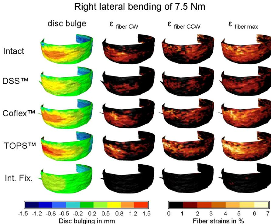
**Fig. 7.** Right lateral bending was applied to specimens in a non-treated condition and after the DSS™, Coflex™, internal fixator (Int. Fix.) and the TOPS™ were inserted. These conditions were evaluated by means of disc bulging, clockwise ( $\epsilon_{CW}$ ), counterclockwise ( $\epsilon_{CCW}$ ) and the ( $\epsilon_{max}$ ) fiber strains. An oblique front view is shown.
