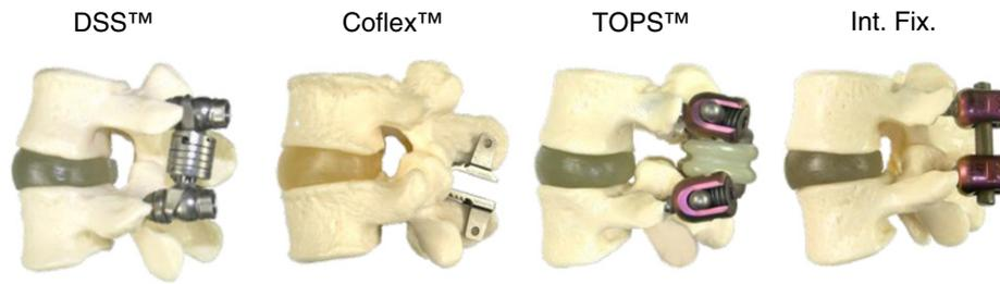
**Fig. 2.** Three different posterior motion preserving implants were evaluated and compared to the non-treated condition. Furthermore, an internal fixator was utilized to mimic a rigidly fixed situation. Following implants were considered: DSS™, interspinous implant Coflex™, a total facet joint replacement (TOPS™) and an internal fixator (Int. Fix.).
