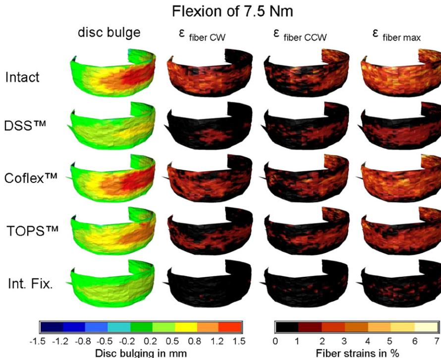
**Fig. 4.** Oblique front view at four different implants and the intact condition were analyzed when the specimens were bended in flexion. This figure shows disc bulging and fiber strains ( $\epsilon$ ) in clockwise (CW), counterclockwise (CCW) and both (max) directions.
