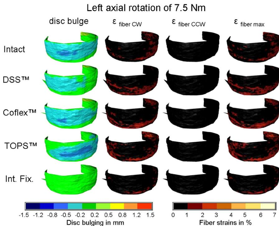
**Fig. 8.** Four different implants and the intact condition were analyzed when the specimens were exposed to torsional moments producing left axial rotation. This figure delineates disc bulging, clockwise (CW), counterclockwise (CCW) and the (max) fiber strains ( $\epsilon$ ).
