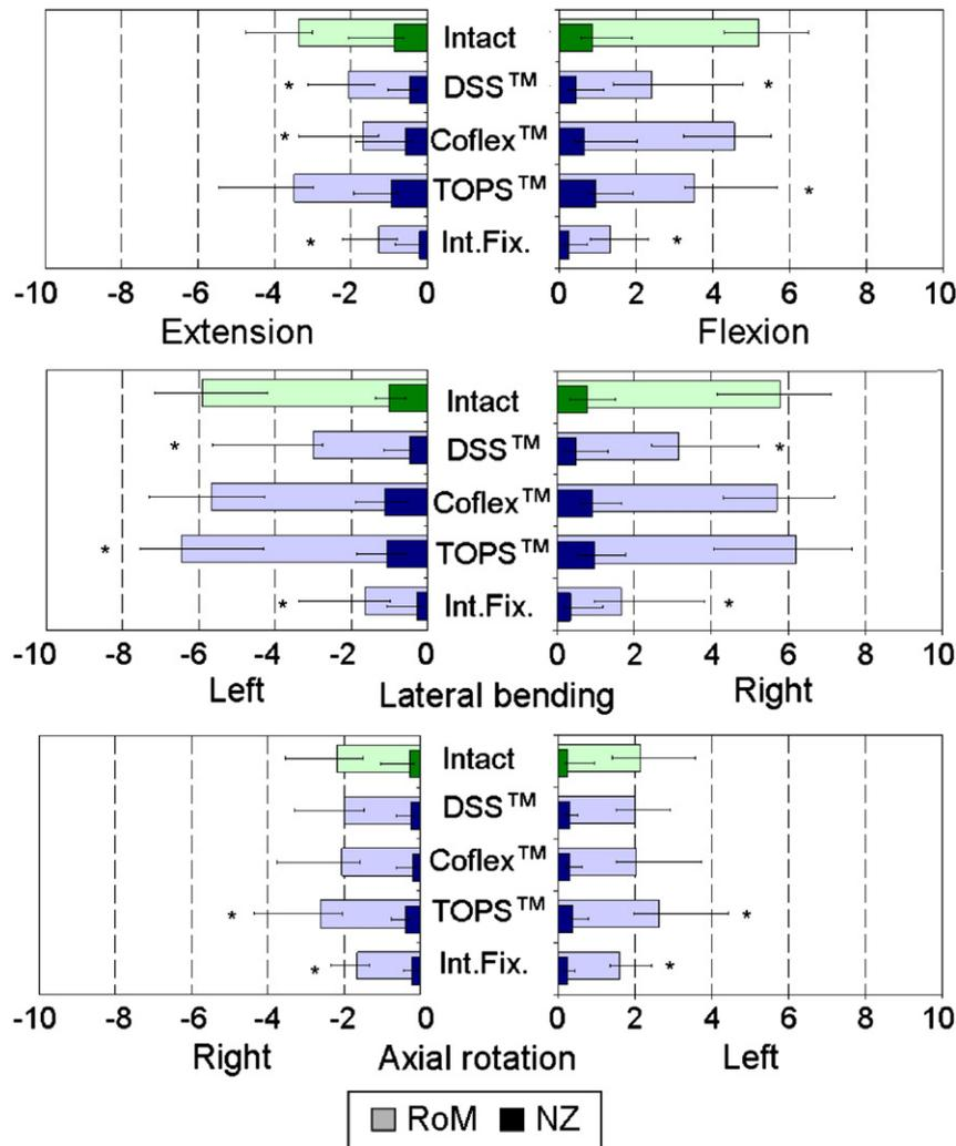
**Fig. 5.** Range of motion (RoM) and neutral zone (NZ) in degrees. Tested were the six specimens in lateral bending, flexion, extension and axial rotation. The four implants were evaluated by means of the RoM and NZ data. (\*) significantly different from the intact condition indicated by the Wilcoxon signed rank test.
