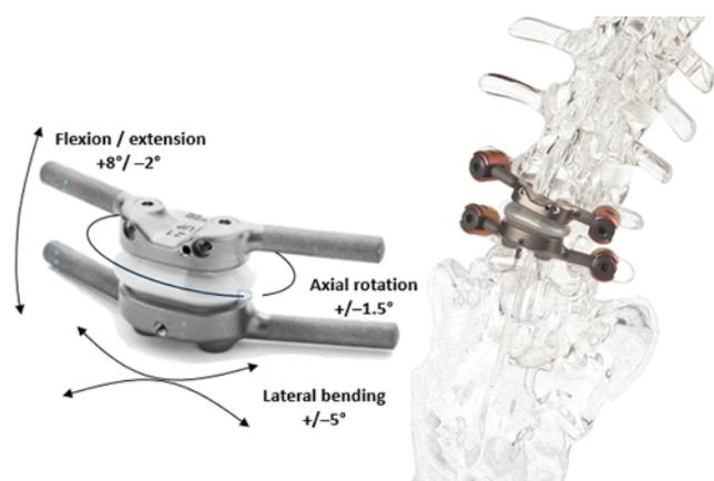
**FIG. 1.** The TOPS device investigated in the current study. The device consists of titanium articulating elements with polyurethane buffers and a polyurethane housing to contain any wear debris. © Premia Spine Ltd., published with permission. Figure is available in color online only.
