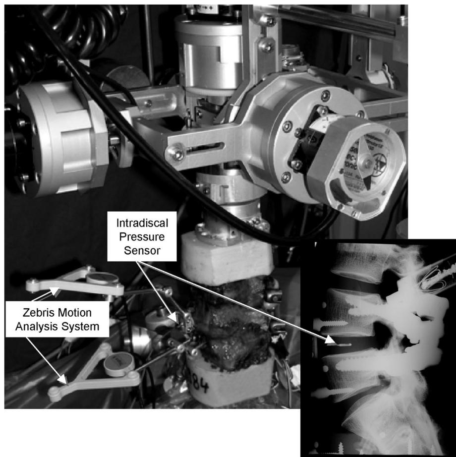
Figure 2. Setup of the experiment in the spine simulator with implanted specimen instrumented with the Zebris motion analysis system (Isny, Germany) and pressure transducer placed in the center of the disc L4–5 (also see radiograph).
