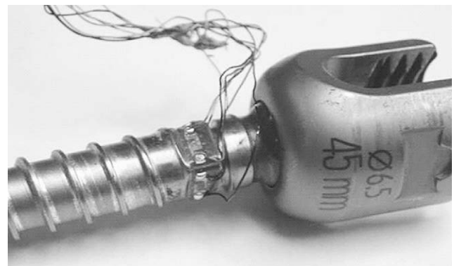
Fig. 4. Four strain gages were attached to the pedicle screws. Data were collected from the pair (180° from each other) with the higher reading after a static load was applied.
