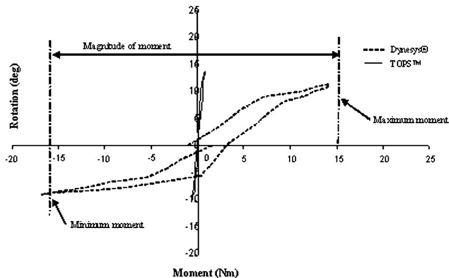
Fig. 5. Representative graph of moment measured in screw 3 plotted against rotation during flexion–extension with a 210 N compressive load. The magnitude of the moment was determined by subtracting the minimum moment from the maximum moment as illustrated.
